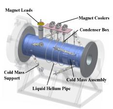
The two spectrometers modules are fully symmetrical. Each is made of a cylindrical tracker immersed into a solenoid field of 4 T.
