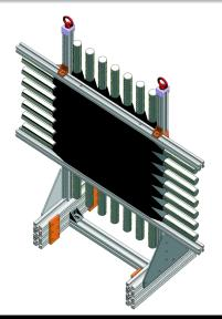
The TOF stations are used for the particle trigger and timing. The timing of each muon allows synchronization to within 50-60 ps with the RF cavity phase. TOF0 and TOF1 are installed in the beamline and TOF2 - after the second spectrometer.
