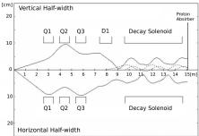
This section is designed to capture as large a pion acceptance as possible from the target, and to select the pions into the decay section. The decay solenoid then serves to accumulate as large a flux of muons as possible.
