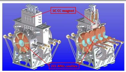
RFCC module has four 201 MHz normal-conducting RF cavities and one superconducting coupling coil (solenoid) magnet. Each RF cavity has a pair of curved Be windows and it operates in a few Tesla magnetic field at 8 MV/m.
