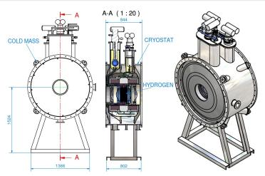
Each muon loses about 12 MeV in the absorber, i.e. 1 W for a beam of  $5 \cdot 10^{11}$  muons per second. The set of two focus coils provides small  $\beta_t$  inside the absorber.
