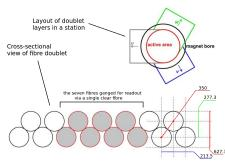
The optical connectors on the station mates seven scintillating fibers to 1.05 mm clear-fiber light guide which transports the light from the stations to an optical patch panel mounted on the end flange of the magnet cryostat. The scintillation light is detected by Visible Light Photon Counters - low band-gap silicon avalanche detectors operated at ~9K.
