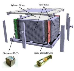
Fully active scintillator calorimeter is located at the very end of the cooling channel. It will stop all muons and electrons and give very distinct signatures for both allowing to measure a muon range. It has the following characteristics:
