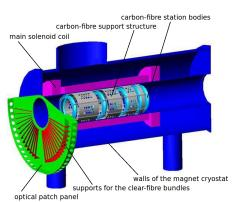
The tracker is made of 5 stations of  $350\mu m$  scintillating fibers perpendicular to the beam axis. The station is made of three planes of fibers rotated by 120°. This allows to reconstruct the full helix track and obtain the momentum.
