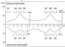
This section consists of a large aperture dipole, to select muons of the desired momentum, and two sets of large aperture quadrupole triplets to transport the muon beam towards the experiment. High-Z (lead) diffuser generates a tunable input emittance.
