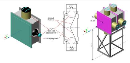
First two CKOVs are installed in the beamline. The Cherenkov light produced in a 2.3 cm thick layer of hydrophobic aerogel is collected by four intersecting conical mirrors reflecting it on four 8" PMTs. Refractive indices of 1.07 and 1.12 are used respectively for the two aerogel planes, ensuring a good muon/pion/electron separation at high momentum: electrons trigger both counters, muons - only one and pions - none.
