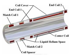
The main solenoid coil is flanked by two correcting coils ensuring field uniformity. Two additional coils on the absorber side provide matching optics with the cooling cell. The three coils are connected in series and are powered by a single 300 amp power supply.
