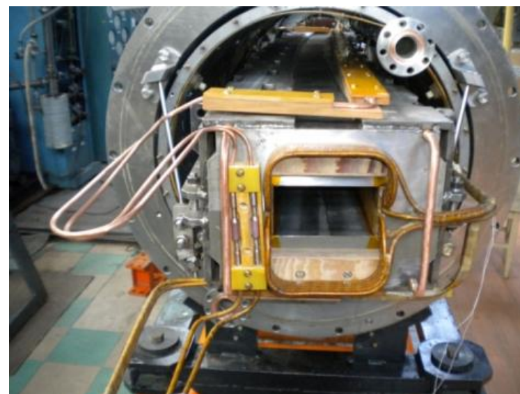
June 2011 SC dipole preparation for the cryogenic test
