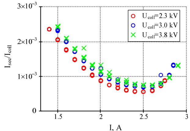
Figure 10: Dependence of efficiency on current in the last coil.
