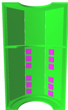
Figure 5: 3D view of magnetic system of Wien filter from Mermaid program.
