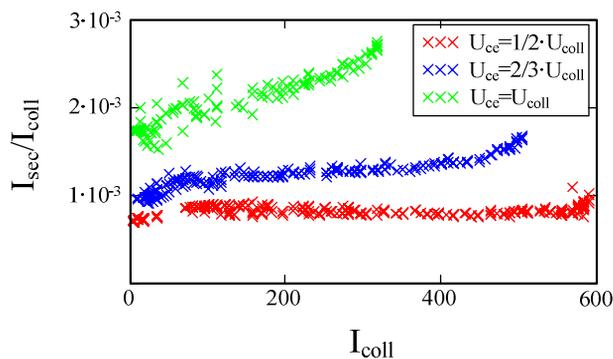
Figure 8: Dependence of efficiency of the collector itself on main beam current.
