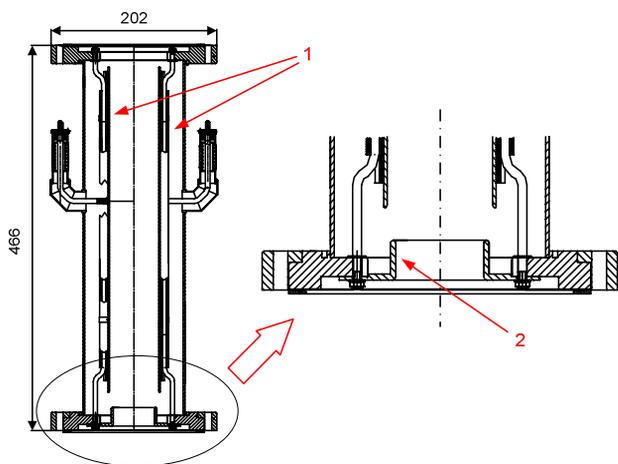
Figure 6: Vacuum chamber of Wien filter.
