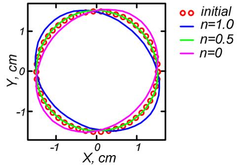
Figure 4: Change of primary beam shape in Wien filter.
