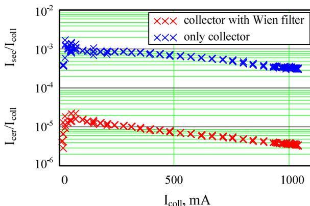
Figure 9: Dependence of efficiency of collector with Wien filter on main beam current.
