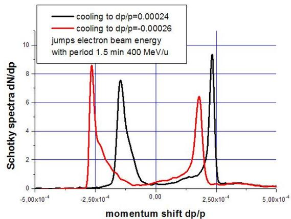
Fig. 13. CSRe momentum spectra of 400 MeV/u carbon beam after procedure of cyclic jump the electron beam energy.
