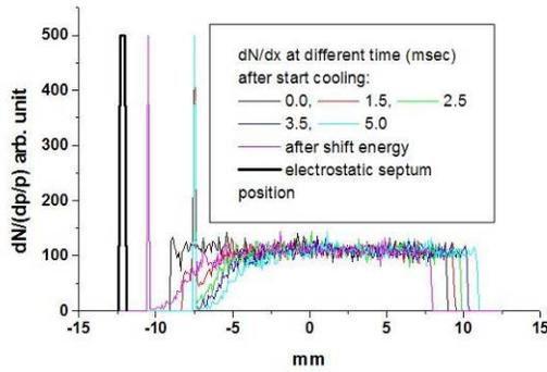
Fig. 9. The 5 msec cycle of carbon ions extraction with electron cooling.
