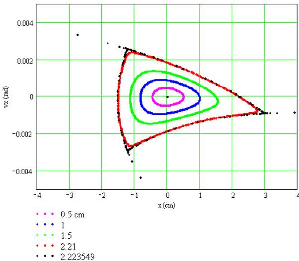
Fig. 4. The computer simulation the horizontal phase plane motion of ions for different initial amplitude with: tune  $\nu_x = 0.36$ , the sextupole value  $\delta = 2 \cdot 10^{-4} \text{ cm}^{-2}$  that introduce nonlinear additional focusing proportional  $1/F = \delta \cdot x$ .
