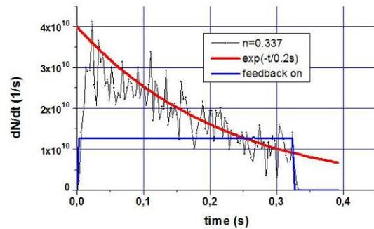
Fig. 6. The computer simulation the electron cooled carbon beam with constant tune and with the feedback for constant extract ion current by modulation the tune storage ion beam..
