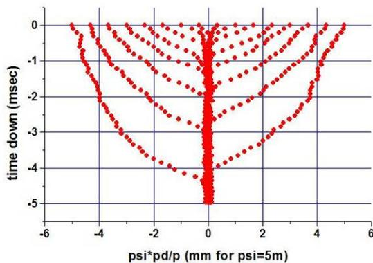
Fig. 8. The computer simulation of initially injected beam cooling (momentum): electron current 0.5 A, electron energy 16 kV, time range arrow is shown from up to down in milliseconds.
