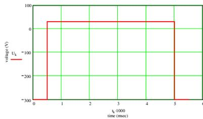
Fig. 10. The voltage on betatron core versus time at cycle.
