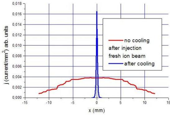
Fig. 3. The transverse profile of the carbon ion beam ( $700 \mu\text{A}$  ( $N_i = 0.44 \cdot 10^9$ )) measured at CSRe.
