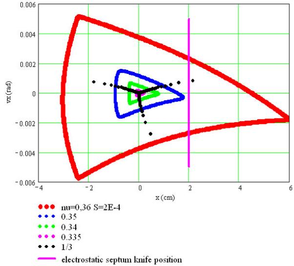
Fig. 5. The profile of separatrix for different horizontal tune.
