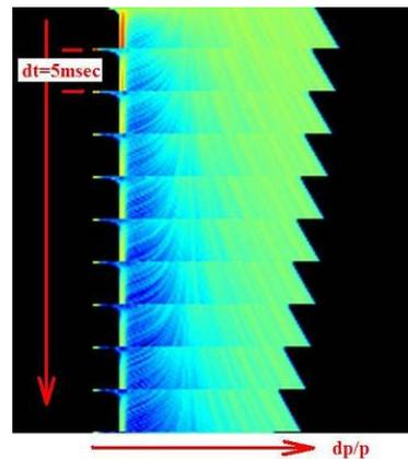
Fig. 12. The computer simulation of 10 cycles of extraction with period 5 msec (full time 50 msec.), initial momentum spread  $\Delta p/p = \pm 0.001$ .
