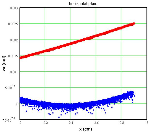
Fig. 7. The horizontal phase plane extracted ion beam. The blue points after pass the focusing lengths at extraction line (vertical scale increased at 10 times).
