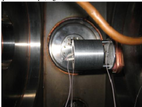
Figure 7. The test electron gun.
