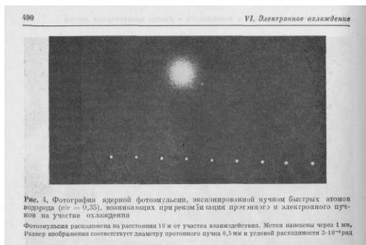
Fig. 14. The first photo of hydrogen atoms beam after recombination at NAP-M cooler [6], distance between mark points 1 mm.
