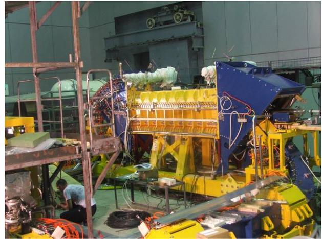
Figure 2: Assembling the 2 MeV electron cooler at BINP.
