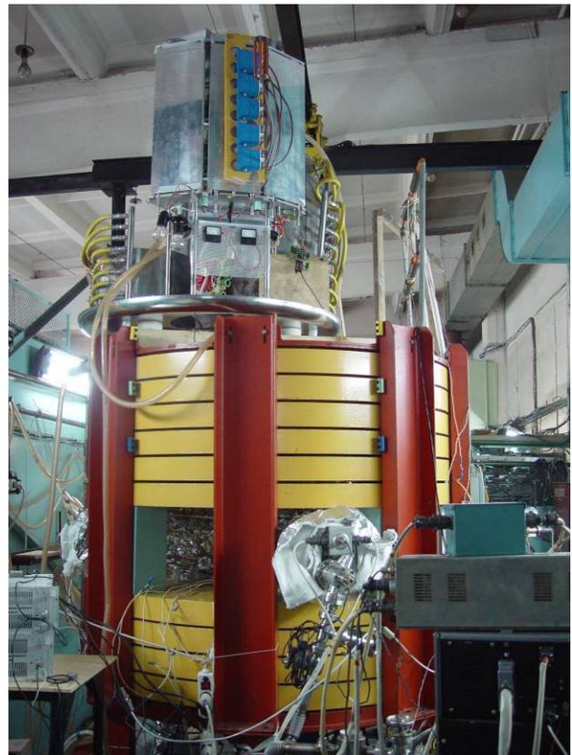
Figure 3: Electron gun and collector test bench at BINP.
