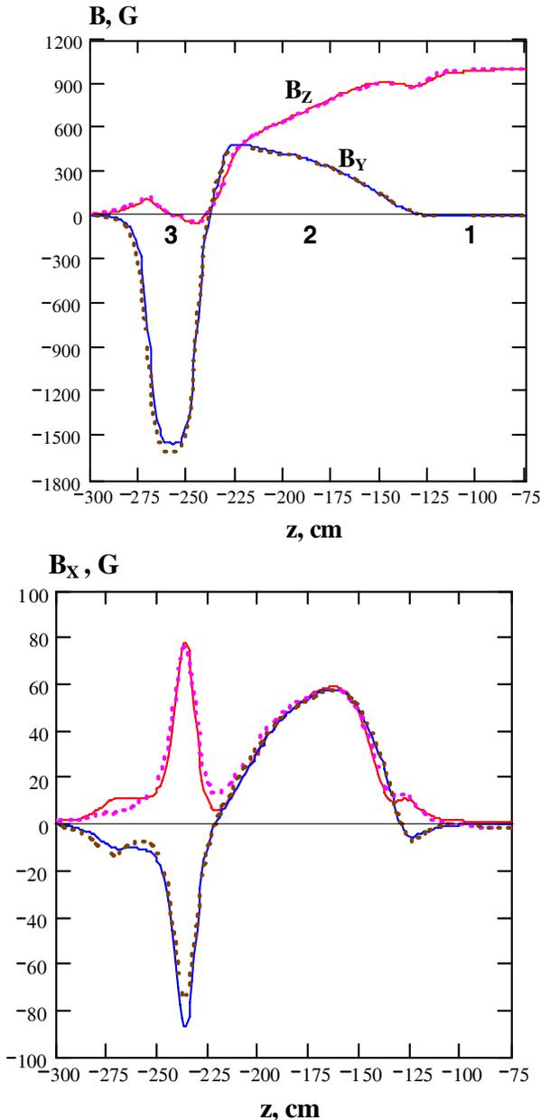
Figure 4: Longitudinal  $B_z$  and vertical  $B_y$  magnetic field components (upper plot) and horizontal  $B_x$  component along two lines with  $x = \pm 2$  cm,  $y = 0$  (lower plot) versus cooling solenoid axis  $z$ . Dots represent measured curves, solid lines- computed curves (MAG3D). The origin is determined in the centre of the cooling solenoid ( $z = -75$  cm). 1-cooling solenoid, 2-toroid, 3-dipole corrector.
