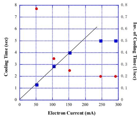
Figure 5: Cooling time and the reciprocal number as a function of the electron current. The clearing voltage is dipole pattern of +/-1 kV.
