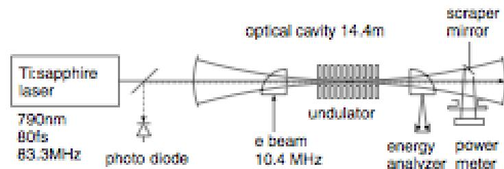
FIG. 2. An experimental setup for a simultaneous measurement of FEL power and absolute cavity length.
