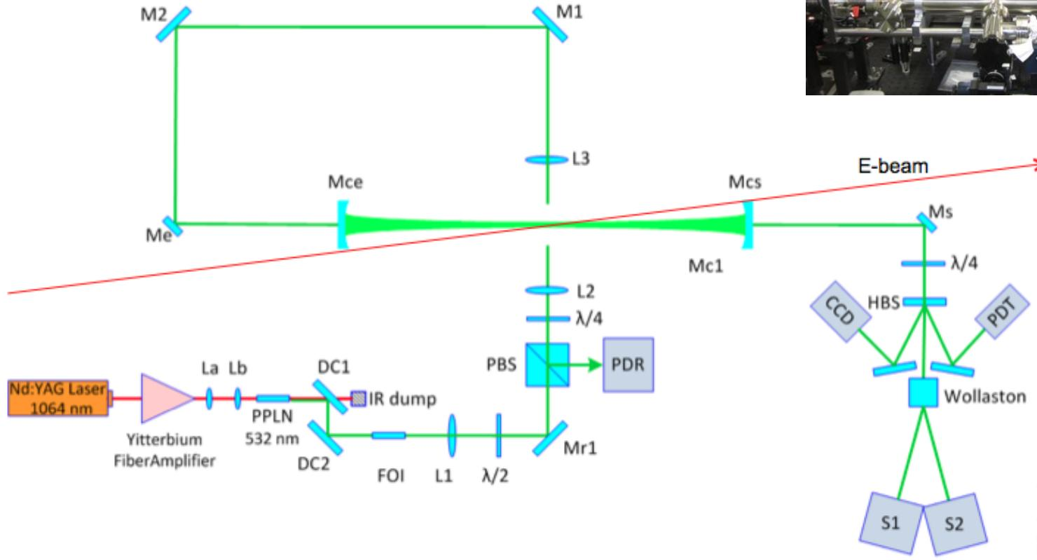
Optical Schematic of HALL A Compton Scattering Laser System
