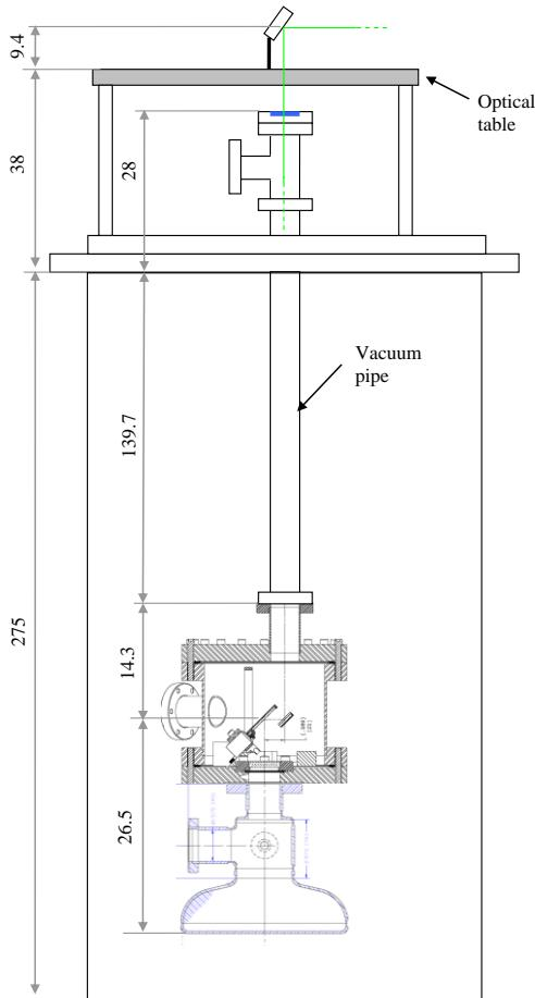
An apparatus was developed to obtain, for the first time, 2D maps of the surface resistance of the inner surface of a superconducting radio-frequency niobium cavity by a low-temperature laser scanning microscopy technique. This allows identifying non-uniformities of the surface resistance with a spatial accuracy of about one order of magnitude better than with earlier methods.
