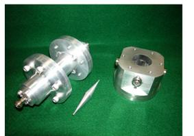
Figure 5. Components of the phase delay measurement test jig with a prototype BPPM
