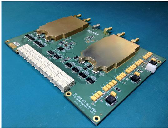
Figure 2: Analog Front End (AFE).
