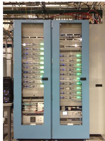
Figure 10: Thermal Test Rack (20-BPMs shown).
