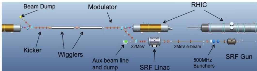
Figure 1: CeC PoP beam line layout. The Modulator, Wigglers and Kicker will be located at the RHIC IR2.
