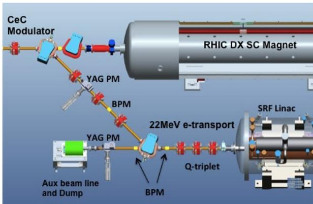
Figure 3: Electron beam diagnostics from the SRF Linac to the CeC modulator.
