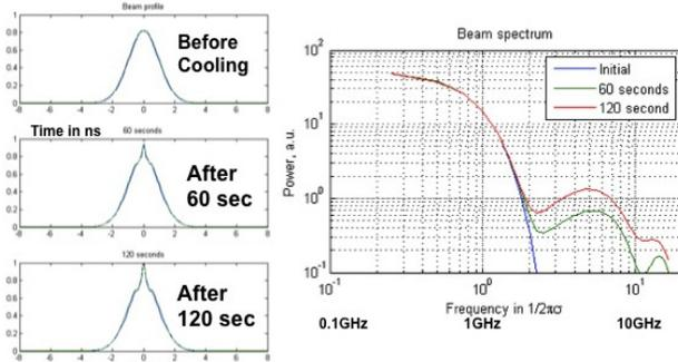
Figure 9: Simulation of RHIC gold 40GeV/n, (rms bunch length 1.5ns) longitudinal bunch profiles during the CeC PoP process with optimal conditions.
