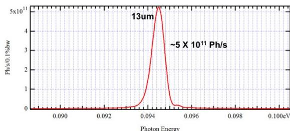
Figure 7: Spectral flux detail of the main harmonic.
