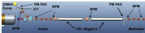
Figure 4: Electron beam diagnostics in the modulator, wiggler, kicker to dump.
