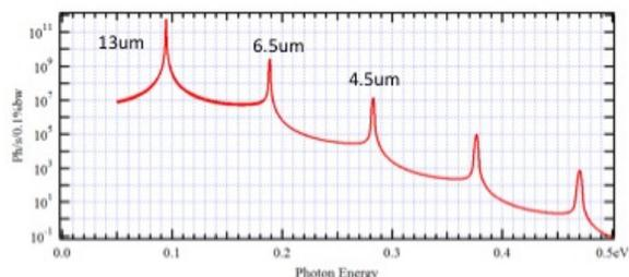
Figure 6: Simulation of spectral flux of spontaneous wiggler radiation using a 100  $\mu$ A e-beam current, normalized rms emittances are 3.3 microns, and relative energy spread is  $3 \times 10^{-4}$ .
