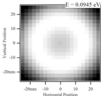
Figure 8: Simulation of the transverse distribution of the optical power 15 m from wiggler. The dip in the middle is due to the spiral electron motion from the helical wiggler.
