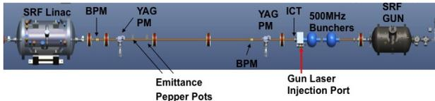
Figure 2: Beam diagnostics in the 2 MeV transport from the SRF Gun to the SRF Linac.
