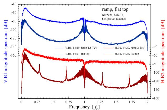
Figure 4: S-BBQ spectra during ramp and squeeze.
