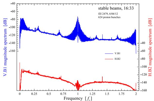
Figure 6: S-BBQ spectra during collisions.
