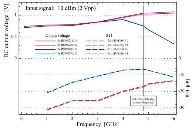
Figure 2: Symmetry of detector output voltages and S11.
