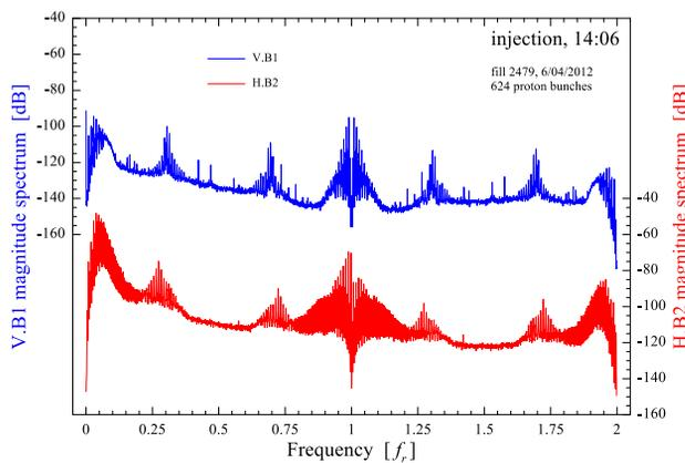
Figure 3: S-BBQ V.B1 and H.B2 spectra at injection.
