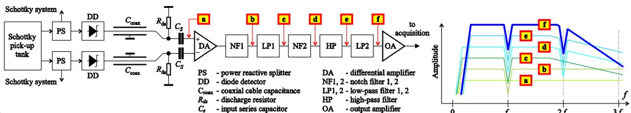
Figure 1: Block diagram of the experimental Schottky BBQ set-up with sketches of the frequency characteristics.
