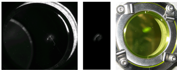
Figure 3: 405nm UV laser spot on YAG crystal in situ.
