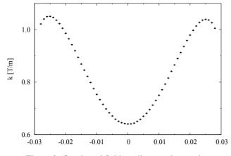
Figure 2: Quadrupol field gradient on the x-axis
