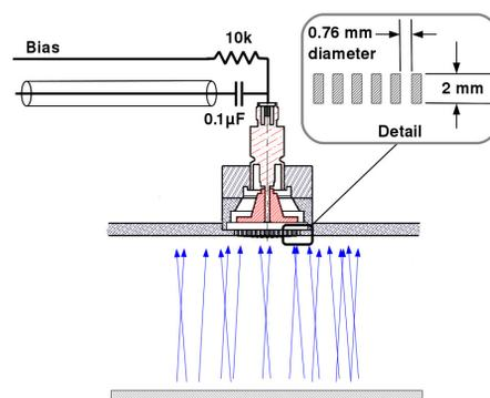
Figure 1: Sketch of Shielded Pickup (SPU)
