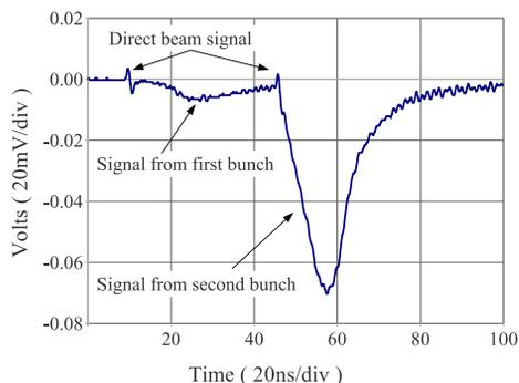
Figure 2: SPU signal with 2 bunches of  $4.8 \times 10^{10}$  positrons each with bunches 36 ns apart. The beam energy is 2.1 GeV
