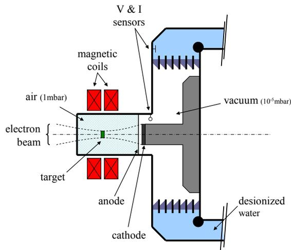
Figure 2: Geometry of the diode.
