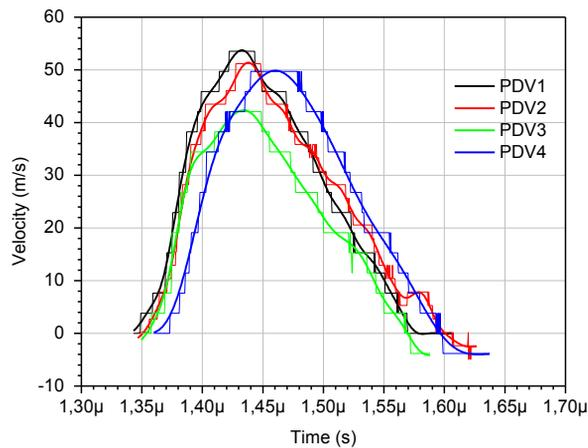
Figure 9: Velocity as a function of time for each of the 4 PDV channels.
