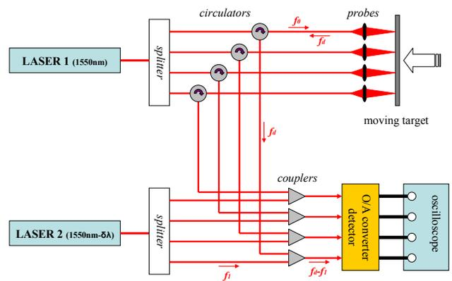
Figure 3: Schematic diagram of the 4-channels PDV set.
