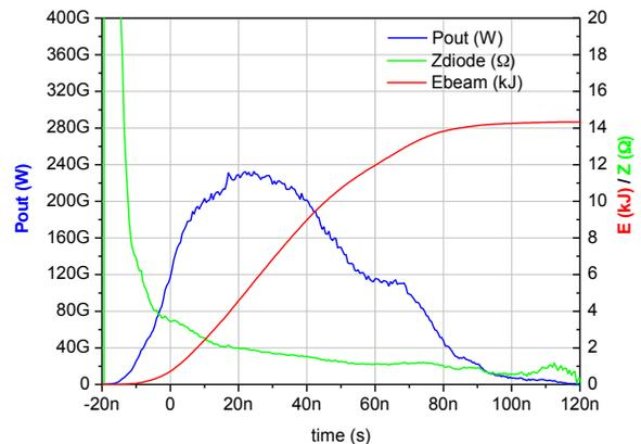
Figure 7: Energy coupling to the electron beam.
