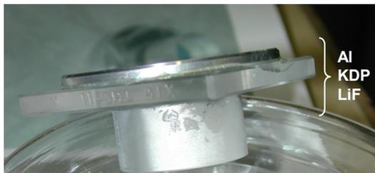
Figure 5. Al/KDP/LiF experimental stack.
