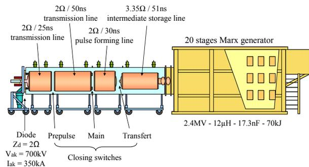
Figure 1: Schematic view of CESAR.
