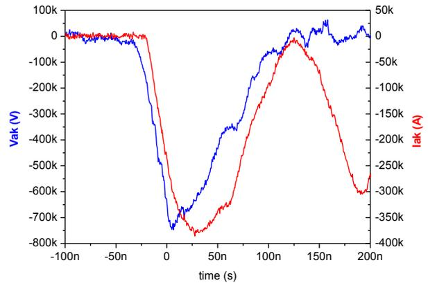
Figure 6: Voltage (Vak) and current (Iak) waveforms on the diode.
