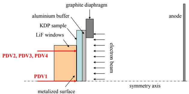
Figure 4: Experimental setup for the KDP crystal test.
