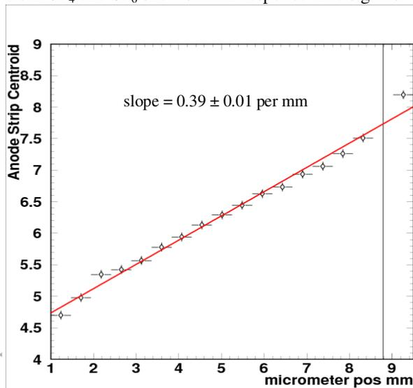
Figure 9. Position resolution beta scan measurements.
