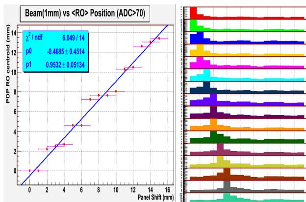
Figure 10: Proton beam position scan with 1 mm aperture.
