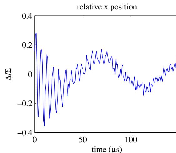
Figure 5: Transverse oscillation of injected beam.
