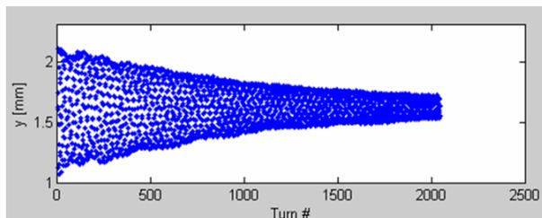
Figure 1: Vertical oscillation amplitudes of stored beam during injection before compensation.
