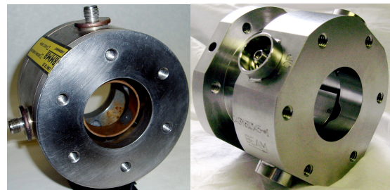
Figure 1: The older BPM (left) shows the inner capacitive Delta-T electrode and a newer BPPM (right) shows a typical inner electrode.
