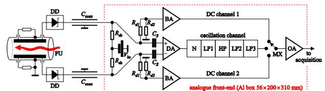
Figure 3: Block diagram of the 3D AFE with detectors.
