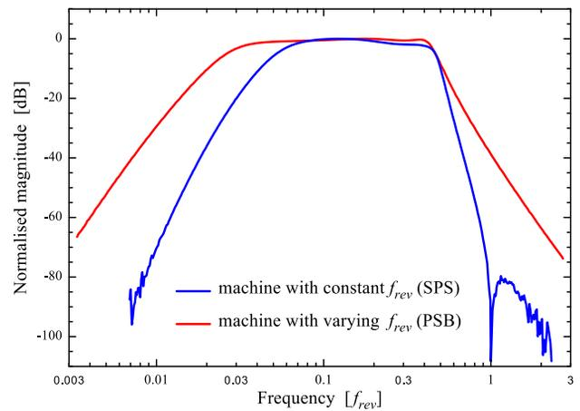
Figure 4: Typical AFE frequency characteristics.
