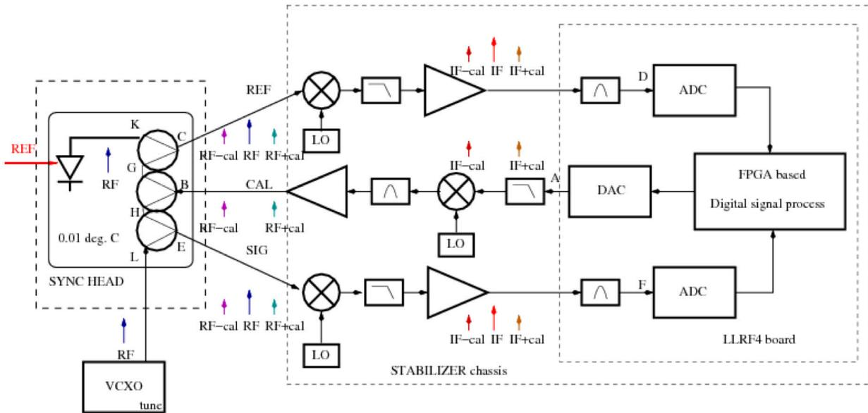
Figure 2: Analog front end circuits.
