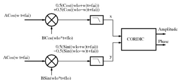
Figure 2: Unit circuit to detect signal phase relative to LO Comb (CIC) filter. The mixer LO port is used to select the spectrum line to be measured. Ideally, only when the  $w=w_{lo}$  does the LPF have nonzero output.
