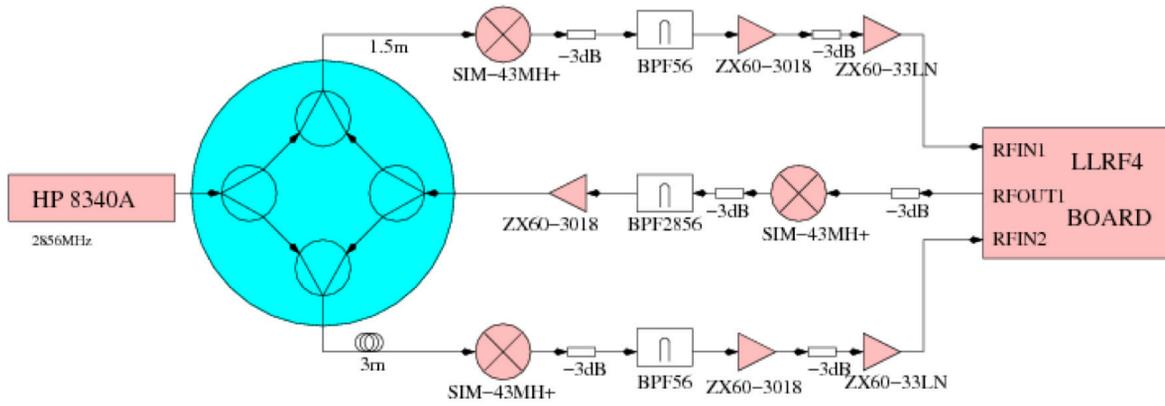
Figure 3: Out of loop test experiment setup.
