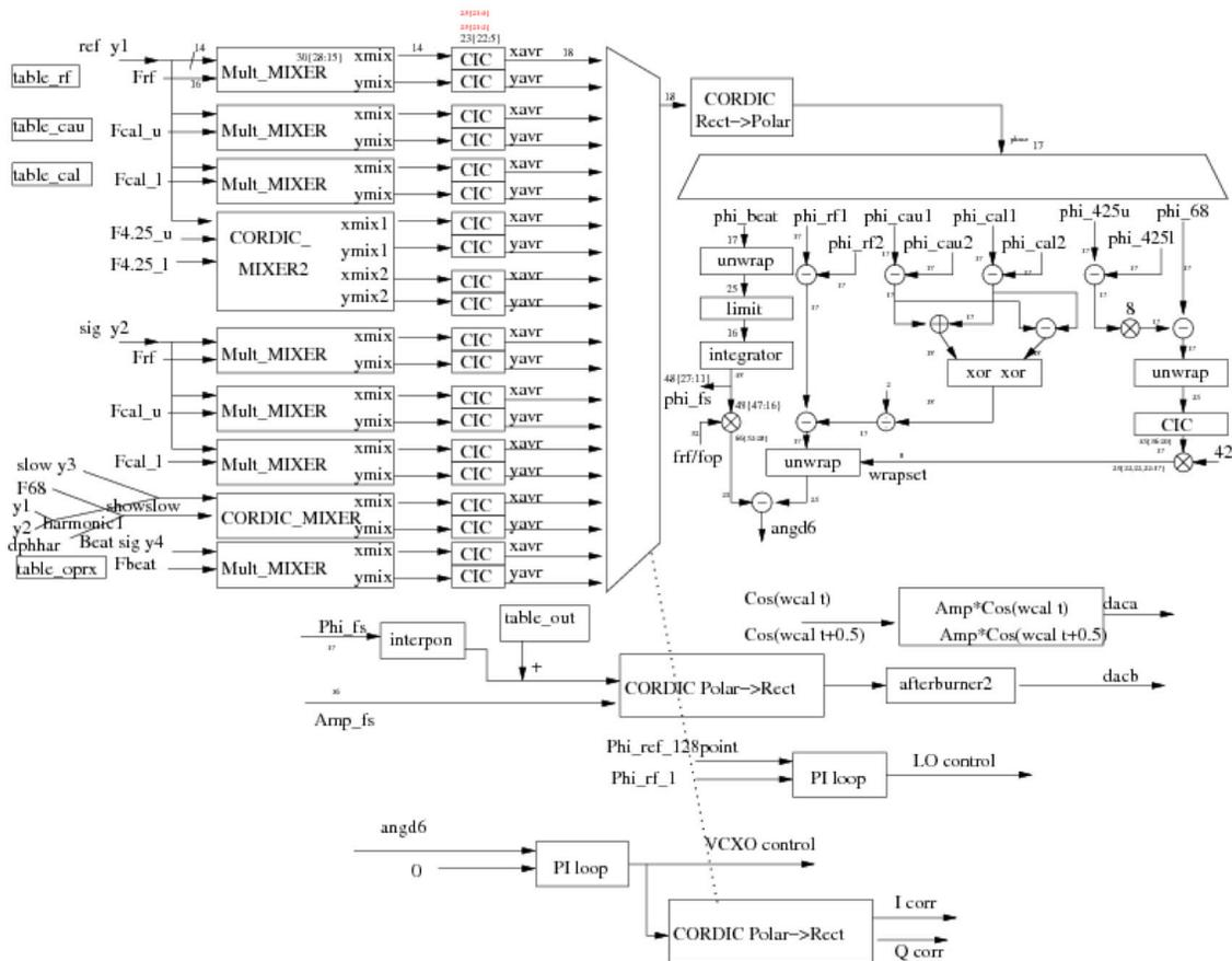
Figure 5: DSP for fs timing distribution system at LCLS.
