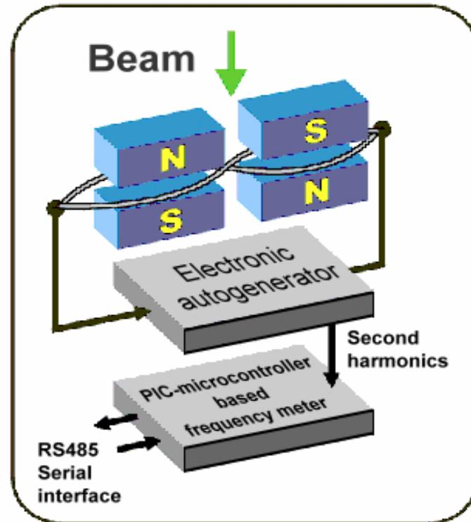
Vibrating wire scanner test in lab
