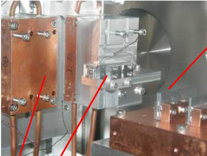
**VWS mounted on the water-cooled plates**
