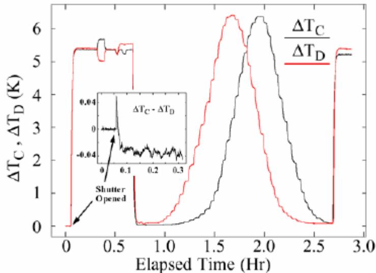
Data collected at a 1-Hz sample rate during a scan of the particle beam's vertical angle in range 100 microradians with 5 microradian steps
