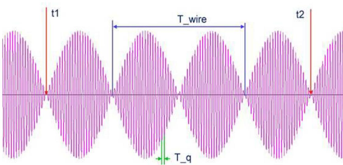
Measurement resolution at  $F_{\text{wire}}$  about 5000 Hz and  $F_{\text{q}} = 1.0000$  MHz
