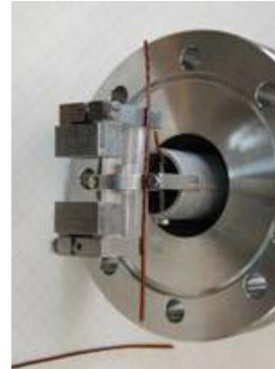
**VWS mounted on tube with below and step motor**
