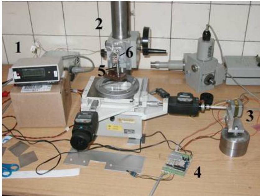
**Laser beam scan experiment layout. 1- Commbox measurement unit, 2 – measuring microscope, 3 – stepper motor feed system, 4 – stepper motor control board, 5 - laser, 6 - VWM**
