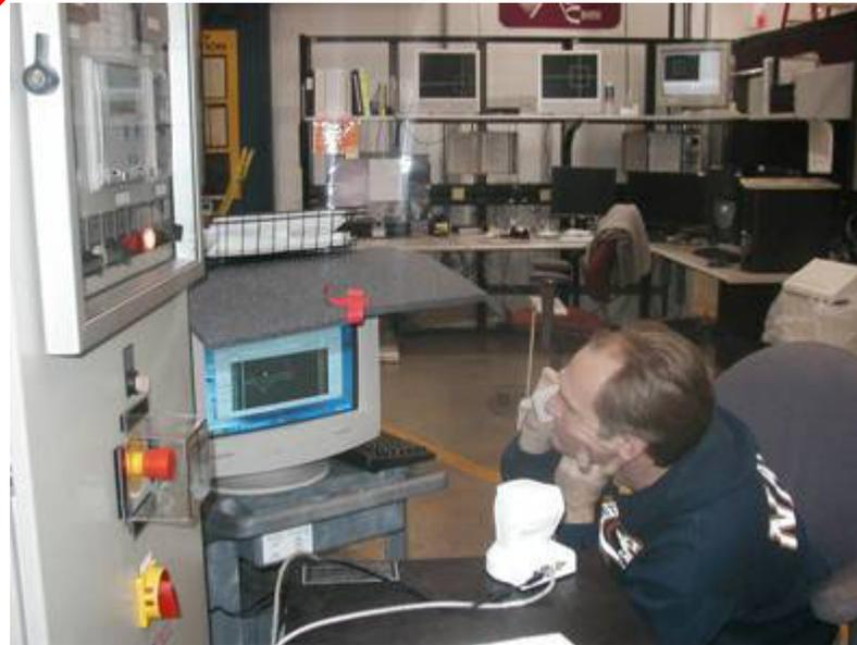
**Alignment procedure to assure that both wires were symmetrically placed above and below the midplane with a clear line of sight to the source (G.Decker)**
