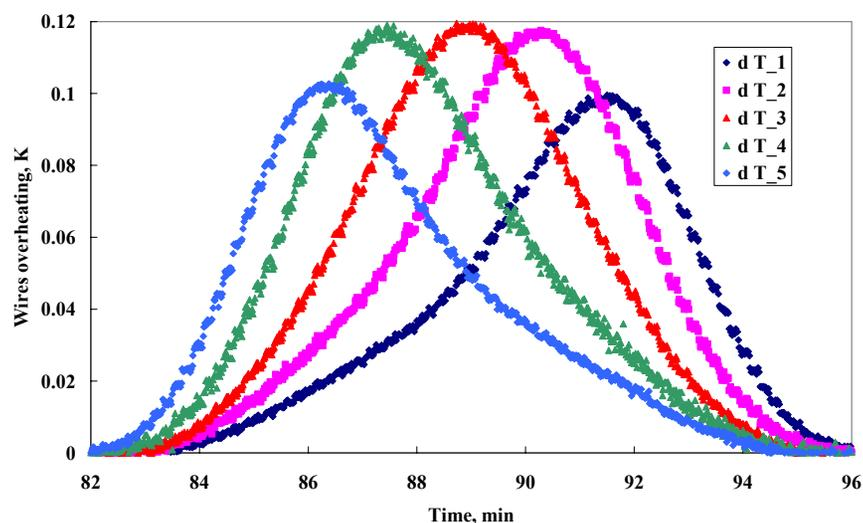
**Scan result presented by wire overheating temperatures. Electron beam was scanned vertically through a range of 300 microradians with 125 steps**
