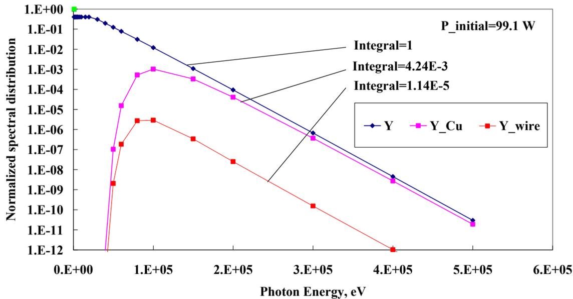
**Normalized spectral distribution of initial synchrotron radiation (Y), passed through the Cu flange (Y\_Cu) and deposited into the wire (Y\_wire). Spectral maximums for Y\_Cu and Y\_wire are about 100 keV**
