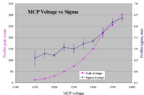
Figure 2. Sigma and peak count vs MCP Voltage
