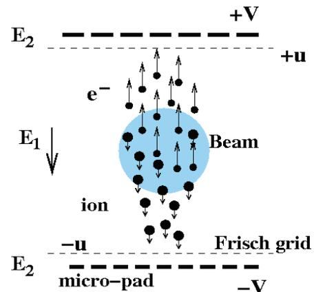
Figure 1: Transverse cross-section of a BTPM. Ionized pairs are sketched in the electric field.
