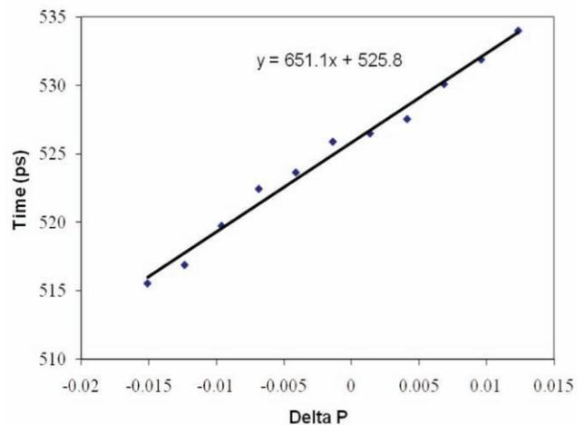
Figure 9: A plot of the change in transit time through the doglegs for different 9-cell rf amplitudes, and hence momentum changes, Delta P.
