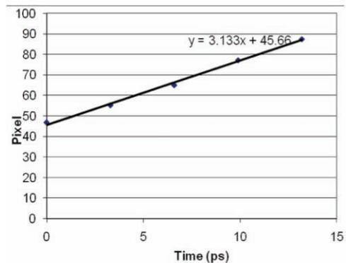
Figure 3: Calibration of the streak camera Range 1 using the laser pulse stacker. The separation of the split laser beam pulses was adjusted with the mirror spacing.
