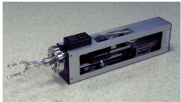
Figure 1. Photo of a new CCL wire-scanner actuator.
