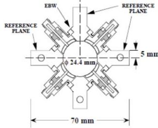
Figure 3: ATF damping ring button BPM.
