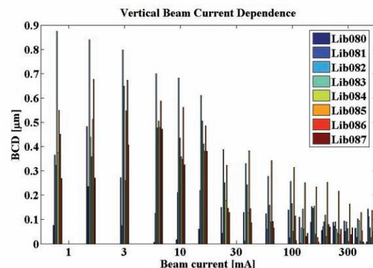
Figure 3: Vertical BCD of 8 Liberations @ 10kHz rate
