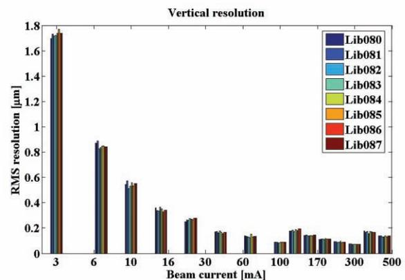
Figure 2: Vertical resolution of 8 Liberations @ 10kHz rate
