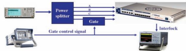
Figure 5: Test setup for latency measurements
