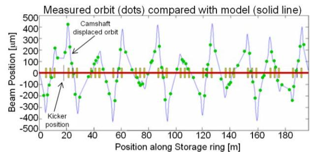
Figure 5: Theoretical and measured camshaft displaced orbit.
