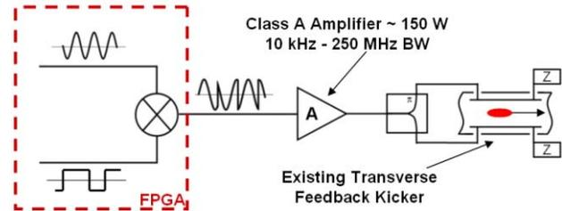
Figure 6: Bunch cleaning system layout.
