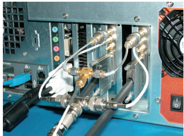
Figure 1: BPPM computer interfaces showing the ZTEC cards (top) and the NI/custom AFE (bottom).
