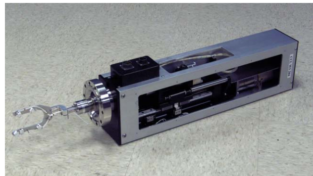
Figure 1. Photo of a new CCL wire-scanner actuator.
