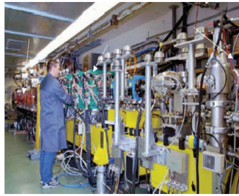
Figure 12: Injection system for CTF3 facility at CERN.
