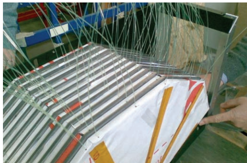
Figure 2: One of the four calorimeters modules during the assembly, wrapped tile, wavelength shifter, and lead plate are clearly visible.
