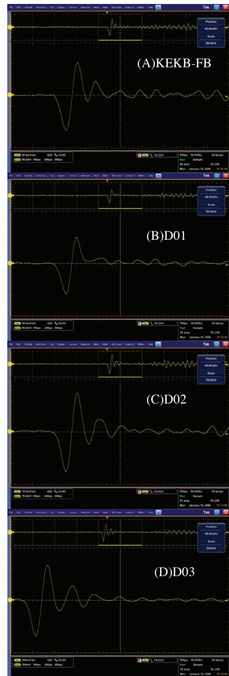
Fig. 19. Beam response of BPMs from linac beam.
