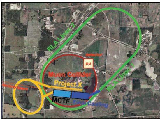
Figure 2: Schematic layout of 1.5–4 TeV Muon Collider on the Fermilab site.
