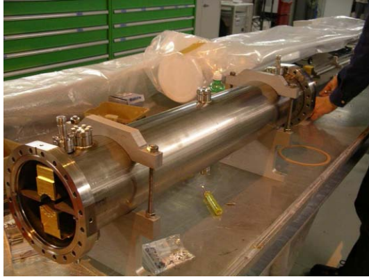
Figure 2: Photo of assembled kicker (Metallic front cap missing)
