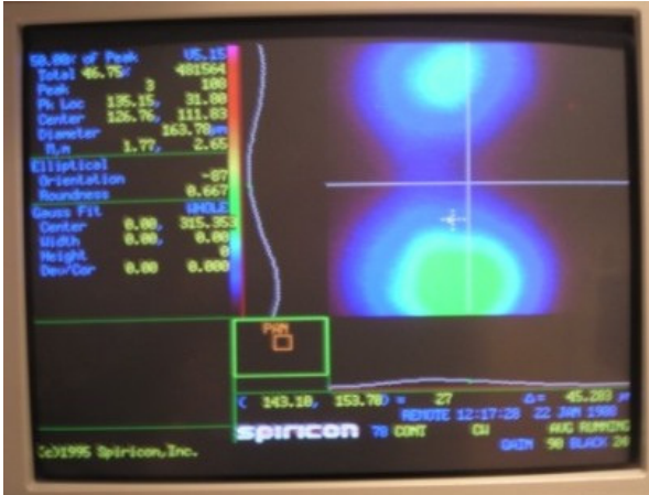
Fig. 5: Synchrotron light image when kicking every other turn.
