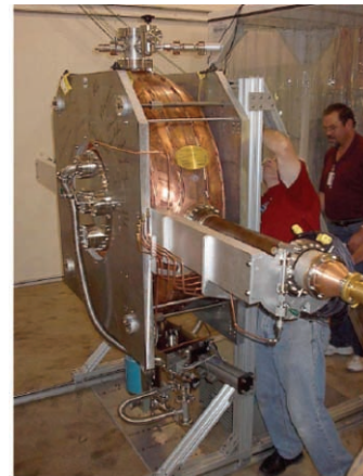
Figure 16: 201-MHz MICE prototype cavity installed in the MuCool Test Area at Fermilab.
