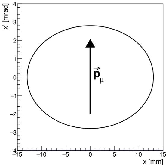
Figure 2: E821  $x$ - $x'$  phase-space admittance in the center of a FODO horizontally defocusing quadrupole magnet. The  $\Delta x'$  is shown for a central momentum pion decaying to a magic momentum muon in the horizontal plane. The signs of  $x'_\mu$  and  $\Sigma^T$  are correlated.
