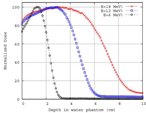
Figure 4: Depth dose curve for 6, 12 and 18 MeV electron beam.
