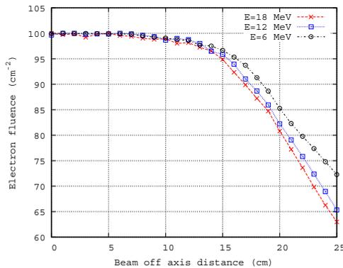
Figure 3: Electron fluence profile along the radius at 100 cm SSD for the optimized primary scattering foil and primary + secondary scattering foil for 6, 12 and 18 MeV.
