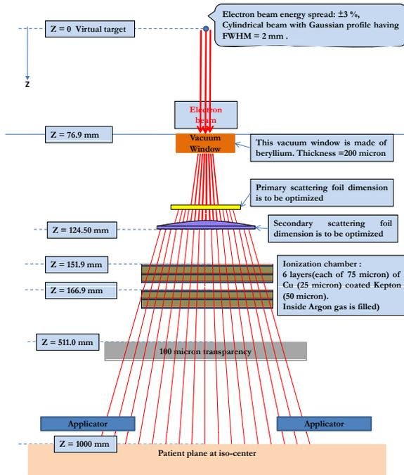
Figure 1: Schematic of the components in accelerator head assembly for electron beam therapy facility.
