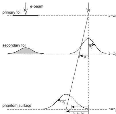
Figure 2: A diagram to define the parameters in the geometry of the dual scattering foil system (left) and the profile of the scattered beam (right).
