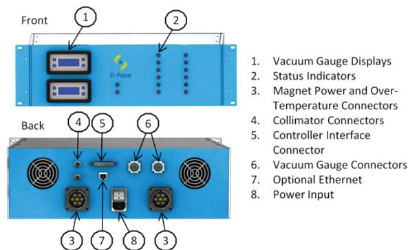
Figure 4: Schematic layout of electronics crate.
