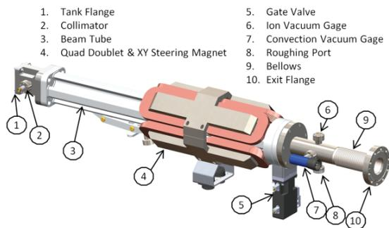
Figure 3: Layout of the mini-Beamline for PET.
