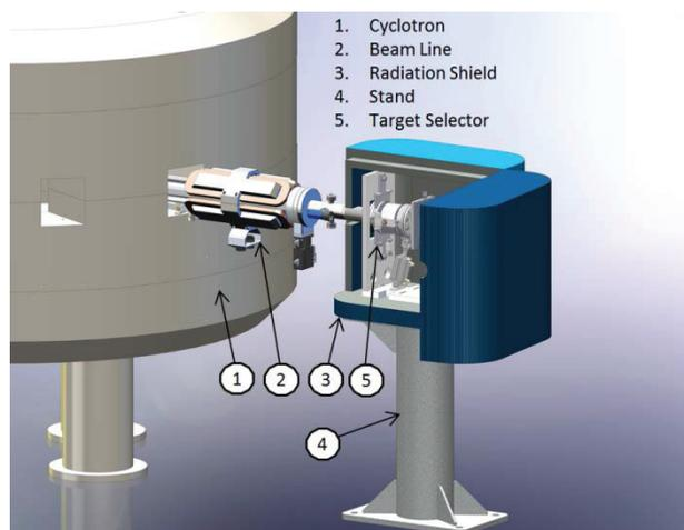
Figure 5: Full beam handling and local-shield for optimized PET radioisotope production on IBA Cyclone®18.
