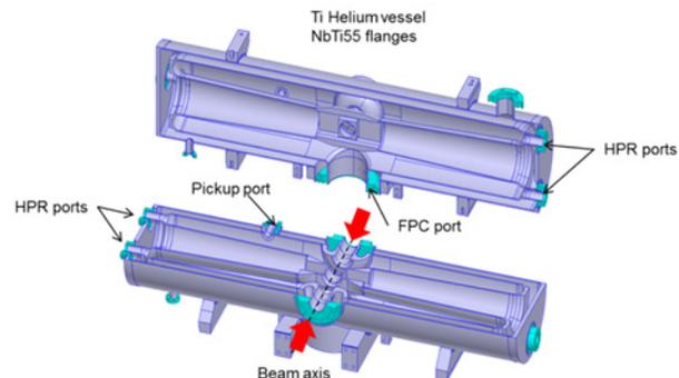
Figure 1: Jacketed HWR cut-view.
