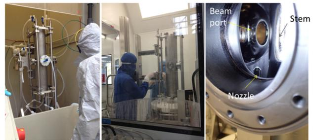
Figure 3: HWR preparation steps at Saclay. From left to right: chemical etching setup, HPWR in ISO5 clean room, view of HPWR nozzle through the FPC port.
