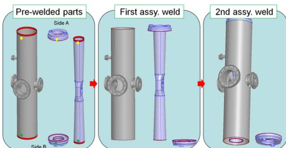
Figure 2: Main HWR parts welding sequence.
