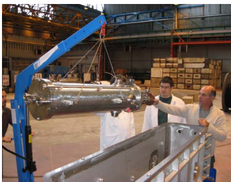
Figure 2: Pre mounting of the cavity in the vacuum tank of the cryomodule. This operation will take place in the CERN clean room.
