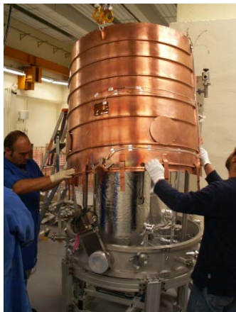
Figure 5: Assembly of the 80K thermal shielding outside the clean room
