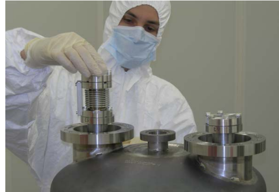
Figure 6: Mounting of the movable plunger on the top of the qualifying cavity.
