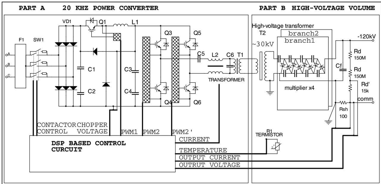
Fig.1. The high-voltage source block-diagram.
