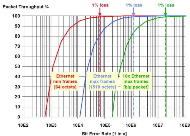
Figure 1: Bit Error Rate in GbE.
