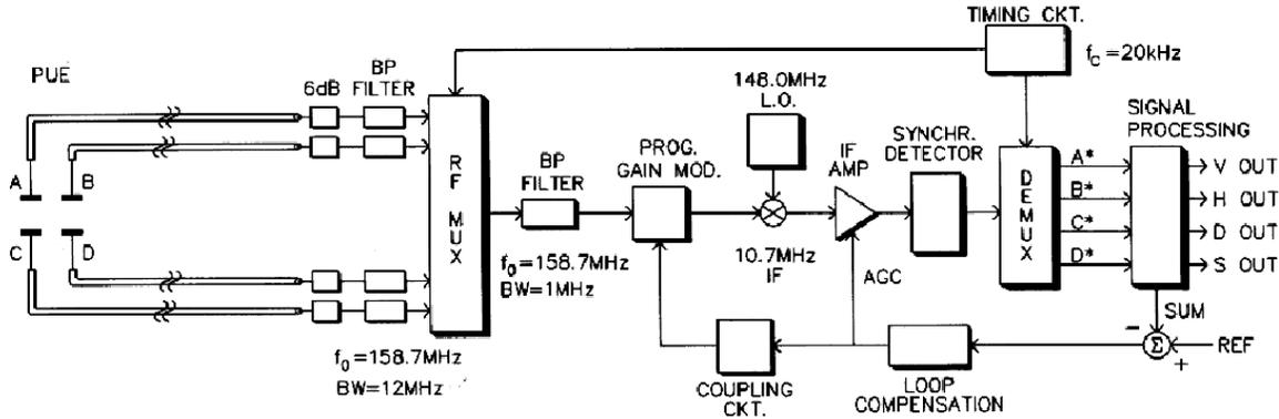
Fig.1. Block diagram of the upgraded BPM
