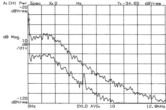
Fig. 4. BPM output noise spectrum with no input signal (upper trace) and with input power = 0 dBm (lower trace).
