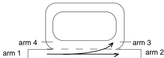
Figure 1: Basic Resonant Ring Circuit
