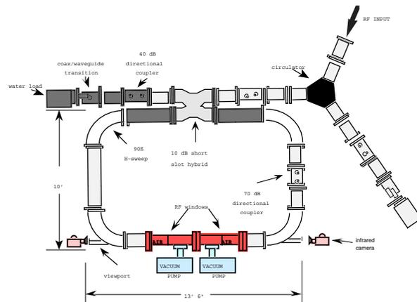
Figure 4: Resonant Ring Test Stand
