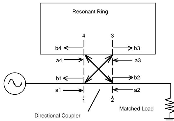
Figure 2: Forward and Reflected Waves in a Resonant Ring Circuit
