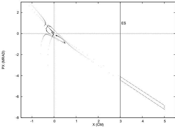
Figure 4: Horizontal phase space at ES during slow extraction at 6 GeV/amu.
