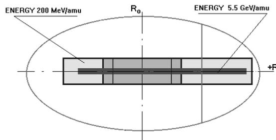
Figure 2: Filling the aperture of the vacuum chamber at a beam energy of 200 MeV/amu and 5.5 GeV/amu.
