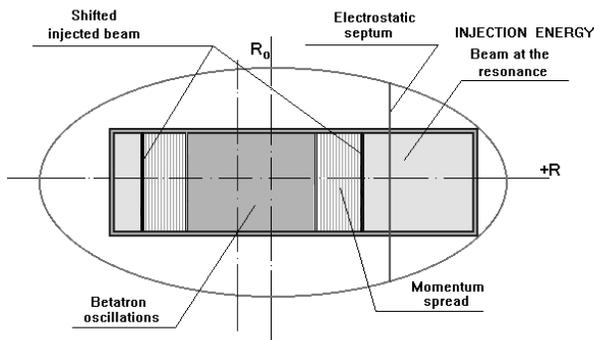
Figure 1: Filling the aperture of the Nuclotron vacuum chamber after the injection at a beam energy of 5 MeV/amu.
