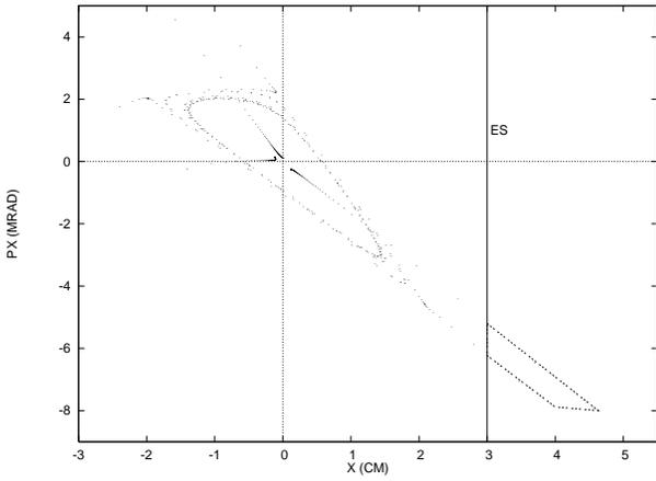
Figure 3: Horizontal phase space at ES during slow extraction at 200 MeV/amu.
