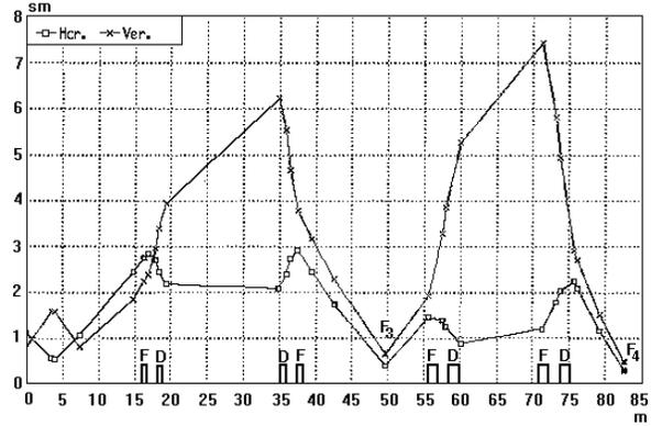
Figure 5: Envelopes of the 200 MeV/amu extracted beam.
