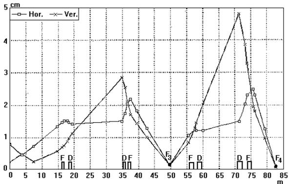
Figure 6: Envelopes of the 6 GeV/amu extracted beam.
