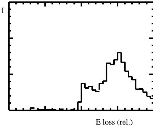
Figure 1: The energy-loss spectrum in aligned crystal of Si(110) simulated for 900-GeV protons with divergence ( $\sigma$ ) of 11.5  $\mu$ rad.
