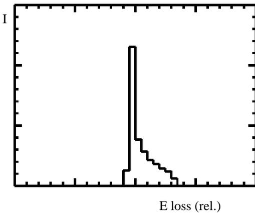
Figure 3: The energy-loss spectrum simulated for parallel protons channeled within  $1 \mu\text{m}$  from the surface of Si(110) crystal.
