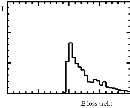
Figure 2: The energy-loss spectrum simulated for a parallel beam of protons in the bulk of Si(110) crystal.
