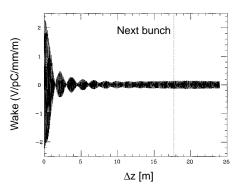
Figure 1: Transverse wakefield as a function of distance  $\Delta z$  for the SLC S-Band structures. The nominal bunch spacing is indicated by the dotted line.
