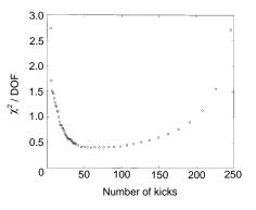
Figure 5: The  $\chi^2$  per degree of freedom as a function of the number of kicks that are included into the solution. About 15 kicks are sufficient to obtain a  $\chi^2/DOF$  of 1.
