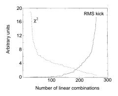
Figure 4: The  $\chi^2$  and the RMS kick found by SVD as a function of the number of linear combinations that are included into the solution. The  $\chi^2$  can be greatly reduced with just a few kick combinations. If too many combinations are included, unphysically strong kicks are introduced that reduce the  $\chi^2$  only slightly.
