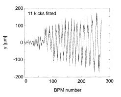
Figure 3: Measured change  $\Delta y_2$  in the electron trajectory due to moving the electron bunch 1 RF bucket (10.5 cm) closer to the positrons. The measurement (solid) is compared to a fit (dashed) for 10 wakefield deflections and an average offset of all structures (compare next section).
