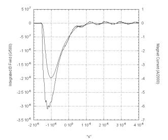
Figure 7. Magnet current and integrated magnetic field.
