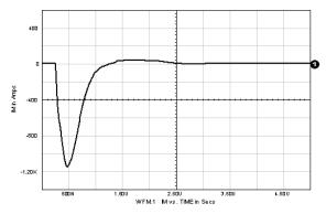
Figure 6. SPICE simulation of the PEP II HER injection kicker system, showing magnet current.
