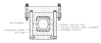
Figure 1. Cross section of the PEP II injection kicker magnet.
