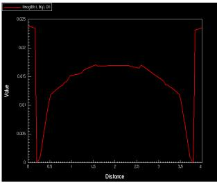
Figure 3. Plot of magnetic field magnitude across the center of the aperture.
