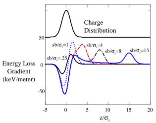
Figure 1. Evolution of the energy loss gradient along the microbunch for 1 nC and a bend radius of one meter. The CSR-induced gradient reaches equilibrium for  $sb/\sigma_z > 6$ . The transient radiation produced when the bunch enters the bend is seen propagating to the right for  $sb/\sigma_z > 4$ .
