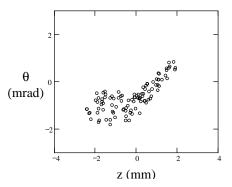
Figure 4. The correlation of divergence with longitudinal position at the exit of the chicane due to CSR.
