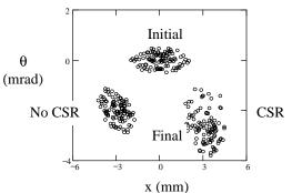
Figure 3. The initial and final transverse phase space distributions, with and without CSR, when the microbunch is compressed. The distributions are offset for display only.
