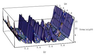
Figure 4: Vertical beam size scan on  $Q_x - Q_y$  plane.
