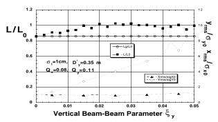
Figure 5: Luminosity and beam size vs.  $\xi_y$  for  $D_y^*=0.35$ m.
