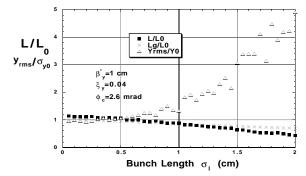
Figure 3: Luminosity and vertical beam size vs.  $\sigma_z$ .
