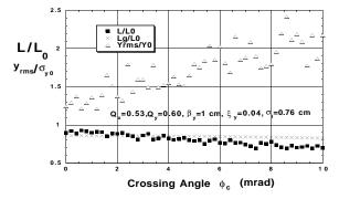
Figure 2: Luminosity and vertical beam size vs.  $\phi_c$ .
