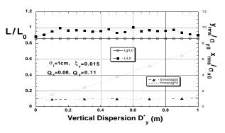
Figure 6: Luminosity and beam size vs.  $D_y^*$ .
