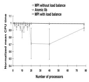
Figure 2: Load balance for the first parallel algorithm. The average CPU-time  $\mu$  is shown as a function of  $N_{proc}$ . The error bars are computed using the standard deviation of the CPU-time for the different processors.
