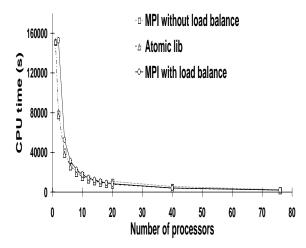
Figure 1: Performance of the first parallel algorithm. The total CPU-time is depicted as a function of  $N_{proc}$ .
