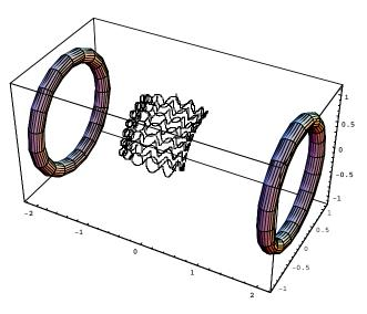
Figure 2: Electron motion in magnetic mirror profile (200 MeV).
