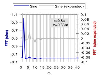
Figure 6: Relative strength of the higher order multipoles at r = 0.8a and z = 0.33.
