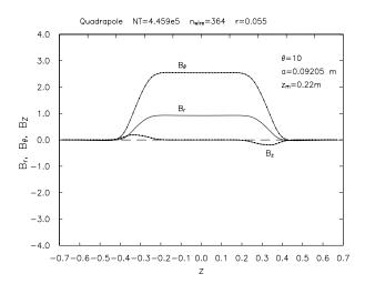
Figure 1: Magnetic Field of the TESLA Quadrupole for r < a
