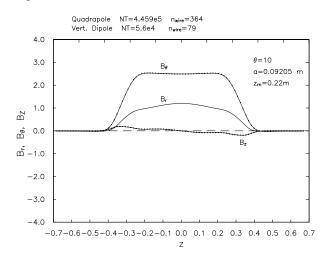
Figure 8: Combined Field of the above Quadrupole and Dipole at r = 0.055 m.
