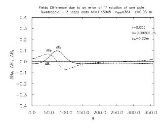
Figure 7: Field errors due to  $1^{\circ}$  shift in the center of one loop
