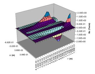
Figure 5: Magnetic Field  $B_z$  of the TESLA Quadrupole along z for 0 < r < 1.5a
