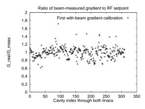
Figure 1: First measurement of linac gradient errors
